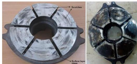
During Start-up and shutdown, however, the thrust bearings are subject to extreme loads with limited or no lubrication.
